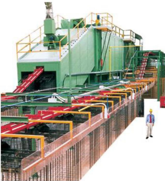
Figure 2: Chrometherm treatment system.
